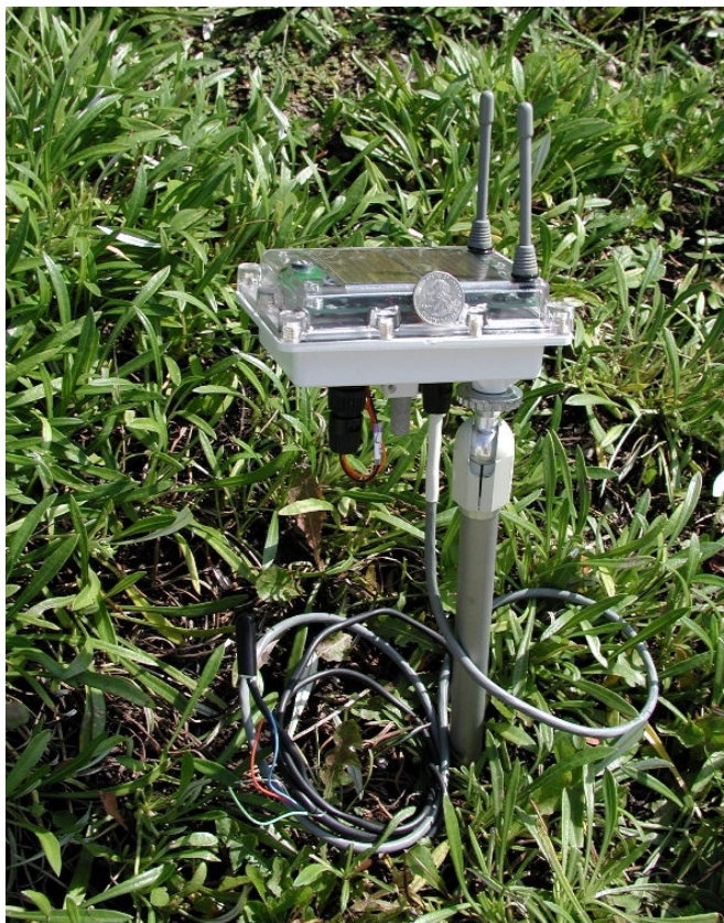
Figure 9. Sensor Web 3 pod. Note the quarter resting on the top. Sensors meant for subterranean measurements (temperature, moisture) can be separately connected as shown.
