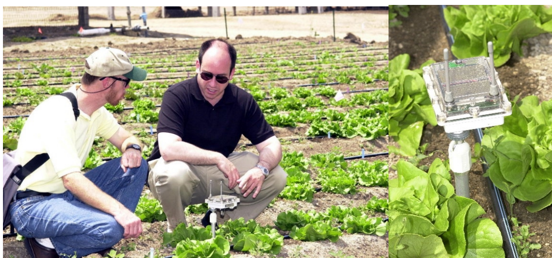
Figure 14. (a) The author (right) and Prof. David Still discuss a Sensor Web 3 pod deployed in a lettuce field. (b) Close-up of pod. Note the dirt and residue on the package.
