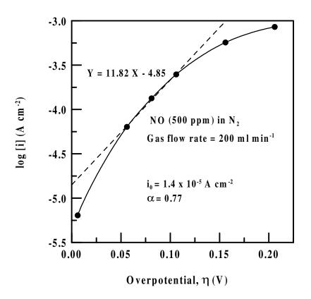
**Figure 6**. A plot of log [i] vs. overpotential in the kinetic controlled region. The slope gives the value of  $\alpha$  and the intercept gives the value of  $i_{0}$ .
