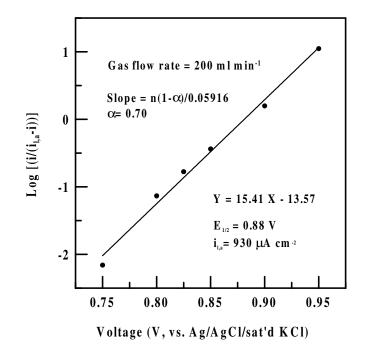
**Figure 5**. A plot of log  $[i/(i_{1,a}-i)]$  vs. E, from which the value of  $\alpha$  can be obtained from the slope and the value of  $E_{1/2}$  from the intercept.
