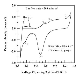
**Figure 2**. Typical cyclic voltammogram (CV or the potentiodynamic current-potential profile) for a Pt/Nafion<sup>®</sup> electrode run in pure  $N_2$  at 20 mV/sec. Solution phase: 0.5 M  $H_2SO_4$ ; The gas flow rate is maintained at 200 ml/min.
