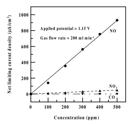
Figure 7. The net limiting current density dependence of NO,  $NO_2$ , and CO concentrations (0-500 ppm) at the same sensing electrode.
