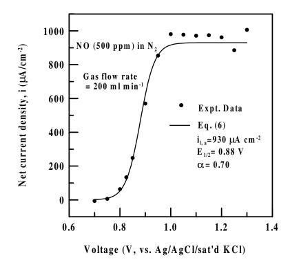
**Figure 4**. The net current density-potential (i-E) data for oxidizing 500 ppm NO at a Pt/Nafion<sup>®</sup> electrode. The gas flow rate is maintained at 200 ml/min. The solid curve is obtained by plotting Eq. (6) with appropriate parameters.
