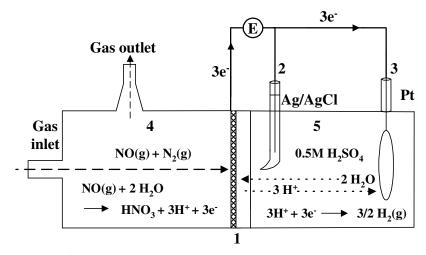
1. WE: Pt/Nafion<sup>®</sup> 2. RE: Ag/AgCl/sat'd KCl 3. CE: Pt disk 4. Gas chamber: NO(g) in  $N_2(g)$  or pure  $N_2(g)$  5. Liquid chamber: 0.5 M  $H_2SO_4$
