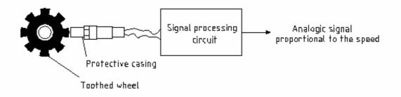
Figure 2. Block diagram of the measurement system.
