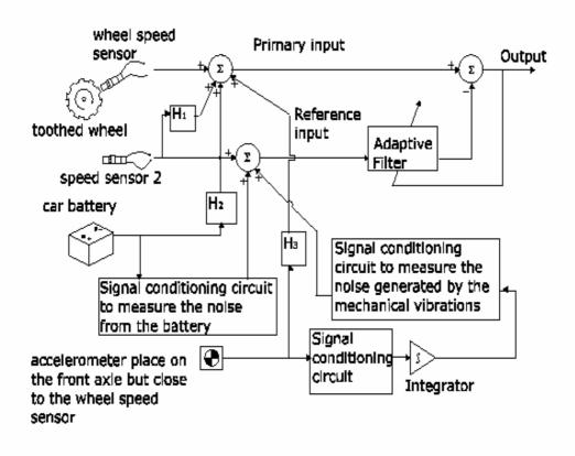
Figure 4. Block diagram of the adaptive noise canceling system.
