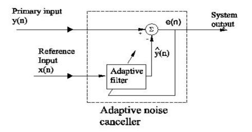
Figure 3. Block diagram representation of the adaptive filter.
