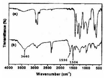
Figure 2. FT-IR spectra of (a) pure PVC and (b) PVC-Polyaniline composite.
