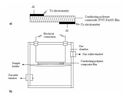
Figure 1. Schematic diagram of (a) electrode and (b) experimental setup used for sensitivity measurements.
