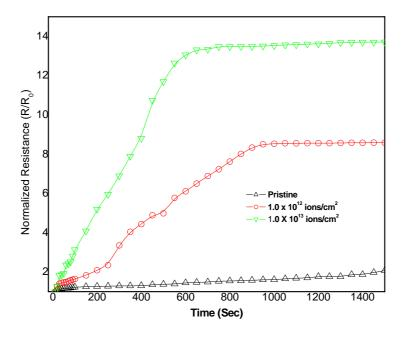
Figure 4. Electrical response of composite films to 1000 ppm of ammonia gas.
