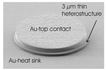
Figure 4. Gunn diode chip: 3µm Gunn-diode heterostructure between two thick Au contacts.
