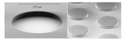
Figure 2. Heat-sink definition with SU-8 resist (left), plated heat-sinks (right).
