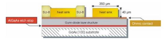
Figure 1. Principle sketch of the first processing steps: heat-sink definition and gold plating.
