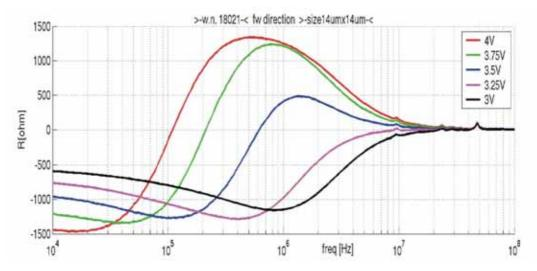
Figure 10. Impedance measurements of a Gunn diode with spacer layers at different supply voltages.
