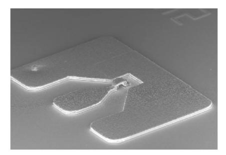
Figure 6. Coplanar layout for S-parameter measurements with air bridge interconnection.
