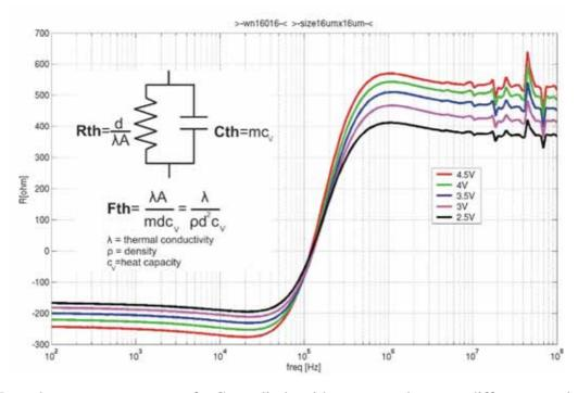
Figure 9. Impedance measurements of a Gunn diode without spacer layers at different supply voltages.
