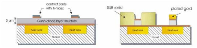
Figure 3. Sketch of the top contact definition, mesa ECR-RIE and top Au plating.
