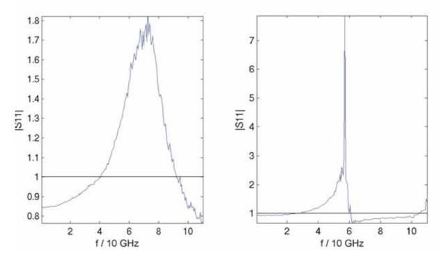
Figure 11. One port S-parameter measurements of the Gunn diode up to 110 GHz: without hot electron injector (left), and with hot electron injector (right).
