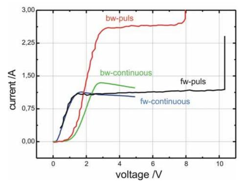
**Figure 8.** Graded gap Gunn diode I-V curve, "bw-puls" and "fw-puls" denotes the backward- (bw) and forward- (fw) directions measured in the 100 ns pulse mode, "bw-continuous" and "fw-continuous" denotes the backward- and forward- directions measured in the continuous mode.
