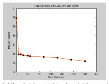
**Figure 9.** 250mm Path Length (134 μm bore size) Response time.
