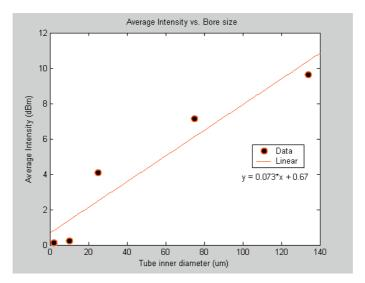
**Figure 4.** Average Intensity vs. Bore size (50 mm path length) at 10 Psi.
