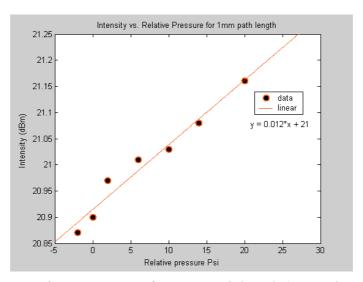
**Figure 7.** Intensity vs. Pressure for 1mm path length (25 μm bore size).
