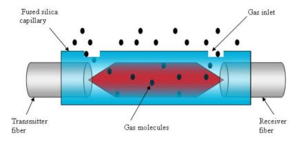
Figure 2. Sample cell gas sensor.
