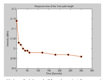
**Figure 10.** 1mm Path Length (25 μm bore size) Response time.
