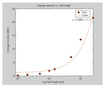
**Figure 5.** Average Intensity vs. Path length (134 μm bore size) at 20 Psi.
