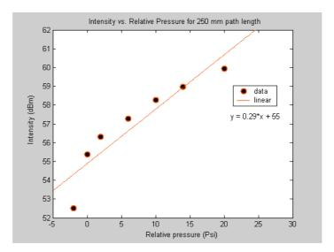
**Figure 6.** Intensity vs. Pressure for 250mm path length (134 μm bore size).
