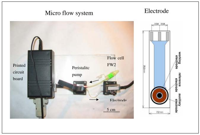
**Figure 4.** The photography of the micro flow system built from the micro pump, flow cell and printed circuit board. The scheme of the designed printed electrodes (working carbon, auxiliary carbon and referent Ag/AgCl electrode).
