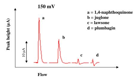
**Figure 5.** A FIA-amperometric record of the naphthoquinones (1 μg.ml<sup>-1</sup>) at the potential of 150 mV. The flow rate of the electrolyte (0.2 M phosphate buffer, pH 5.5) was 0.5 ml.min<sup>-1</sup>. The sample (5 μl) was injected manually. The working electrode was made from glassy carbon, auxiliary carbon electrode and referent hydrogen palladium electrode. For other details see "Materials and Methods" section.
