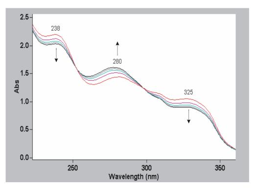
**Figure 6.** The UV spectra of the decomposition of the complex of Mn(III)diacetylacetonehydroxylaminmaleate in ethanol with respect to time (15 min).
