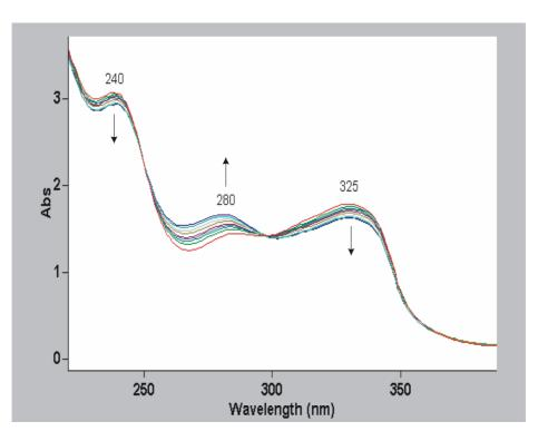
**Figure 4.** The UV spectra of the decomposition of the complex of Mn(III)-diacetylacetonemaleate in ethanol with time (30 min.).
